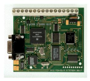
Bitstream GSM-Server BS12 is a complete server equipped with a industrial GSM-modem for wireless connection. The server has a software download feature of code and or parameters within standard software package. Using a standard PC with serial interface, there is no need for separate FLASH programming device.
